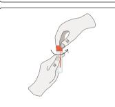
Screw the lid onto the tube tightly to avoid any leakage.
